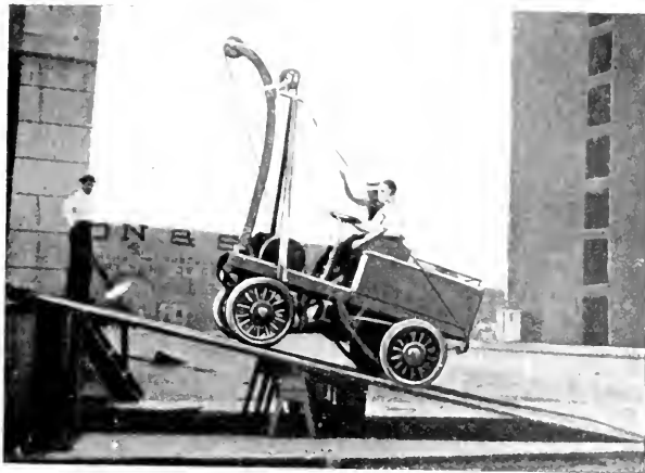
Electric Storage Battery Truck Ascending Incline
